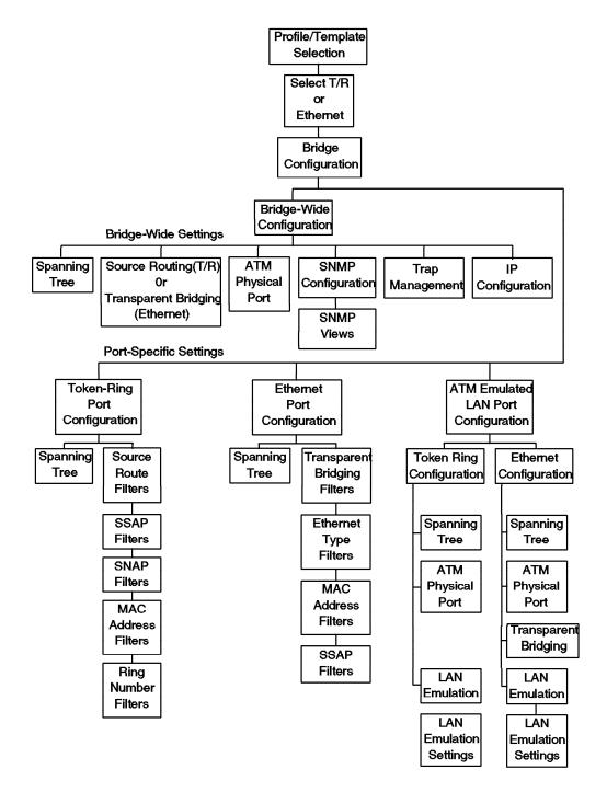
Figure 28. Windows Displayed by the ATM TR/Ethernet Bridge Module Configurator
